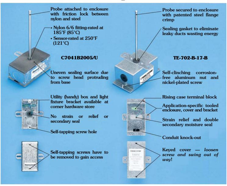
All MAMAC 700 Series Temperature sensors are vibration and shock tested to MIL STD 810, corrosion and lifecycle tested to ASTM B845, Method H. CE, C-Tick, and UL approved. Made in U.S.A.
