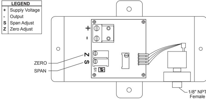
PR-264 pressure transducers with 4–20 mA output units are powered with a 12–40 VDC supply.
