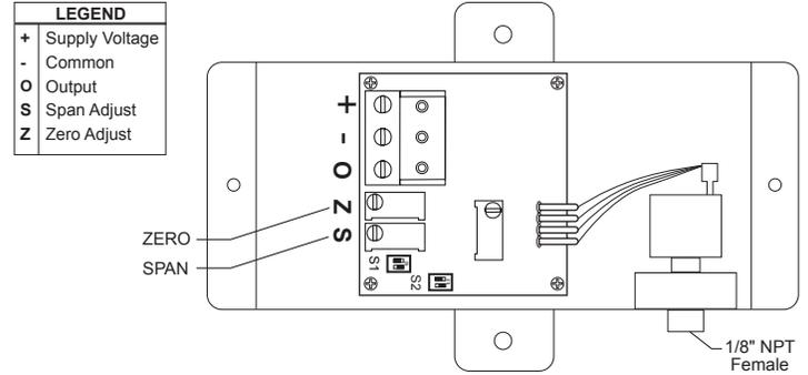
PR-264 pressure transducers with VDC output are field selectable 0–5 VDC or 0–10 VDC output and can be powered with either a 12–40 VDC or 12–35 VAC.
